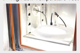
The test equipment opening 4hours, keeping temperature<-40°C, the lamp working fine. The test equipment opening 4hours, keeping temperature>55°C, the lamp keep working fine.
